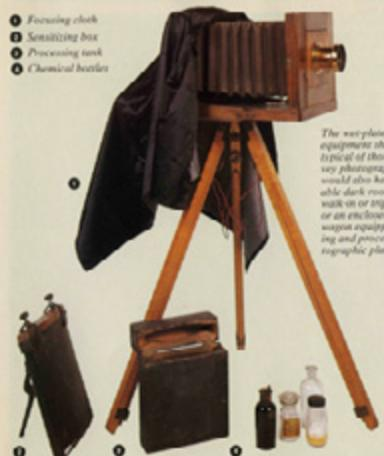
The wet-plate camera and equipment shown here are typical of those used by Survey photographers. They would also have used a portable dark room tent (either walk-in or tripod-mounted) or an enclosed horse-drawn wagon equipped for sterilizing and processing their photographic plates.
